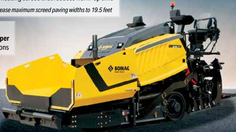
BOMAG’s new 8-foot CR Series 2 paver offers the latest advancements for its highway-class pavers, and the new Versa 16 front-mount screed delivers paving application flexibility.
