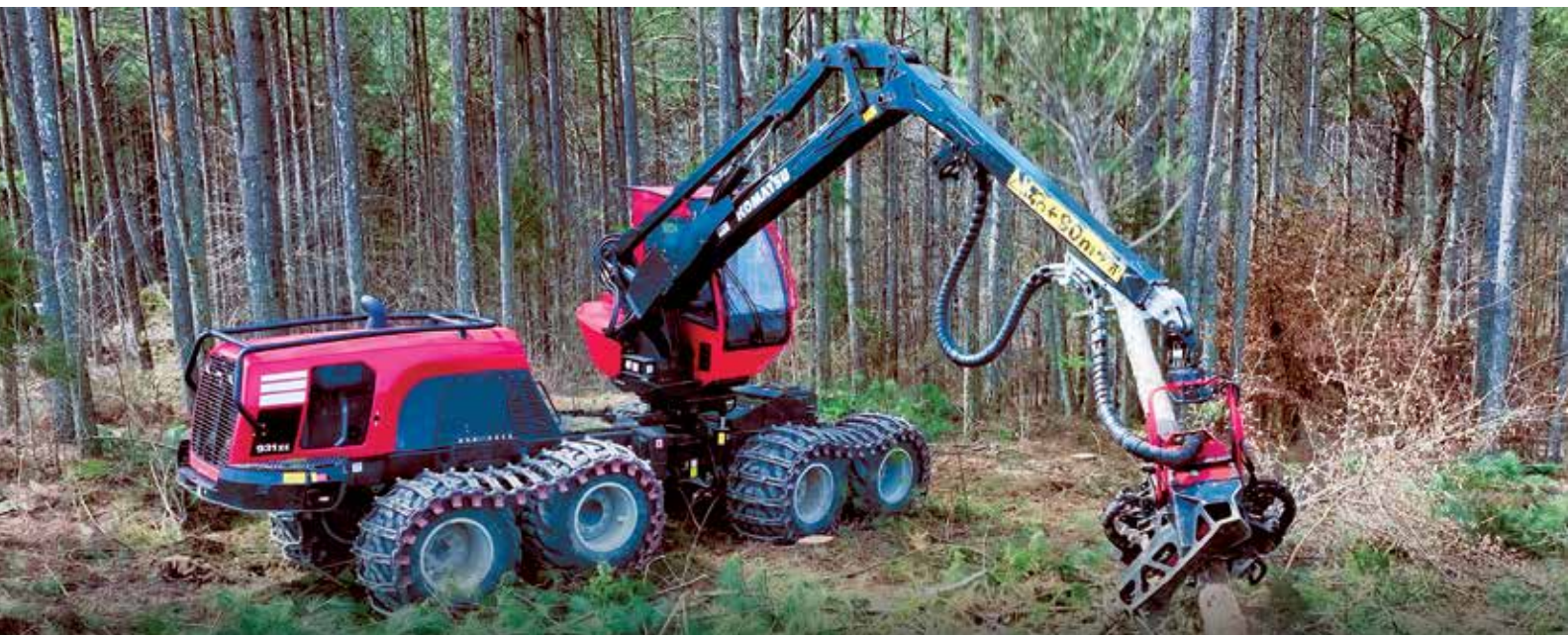
An operator uses a Komatsu 931XC harvester to cut timber to length for a logging operation.
