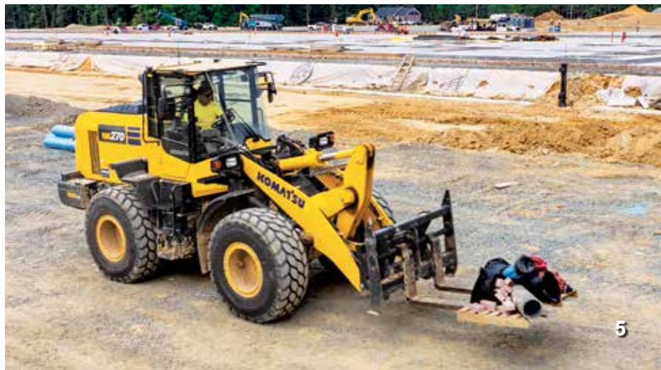
An operator carries various items on a pallet across the jobsite with a Komatsu WA270 wheel loader.
