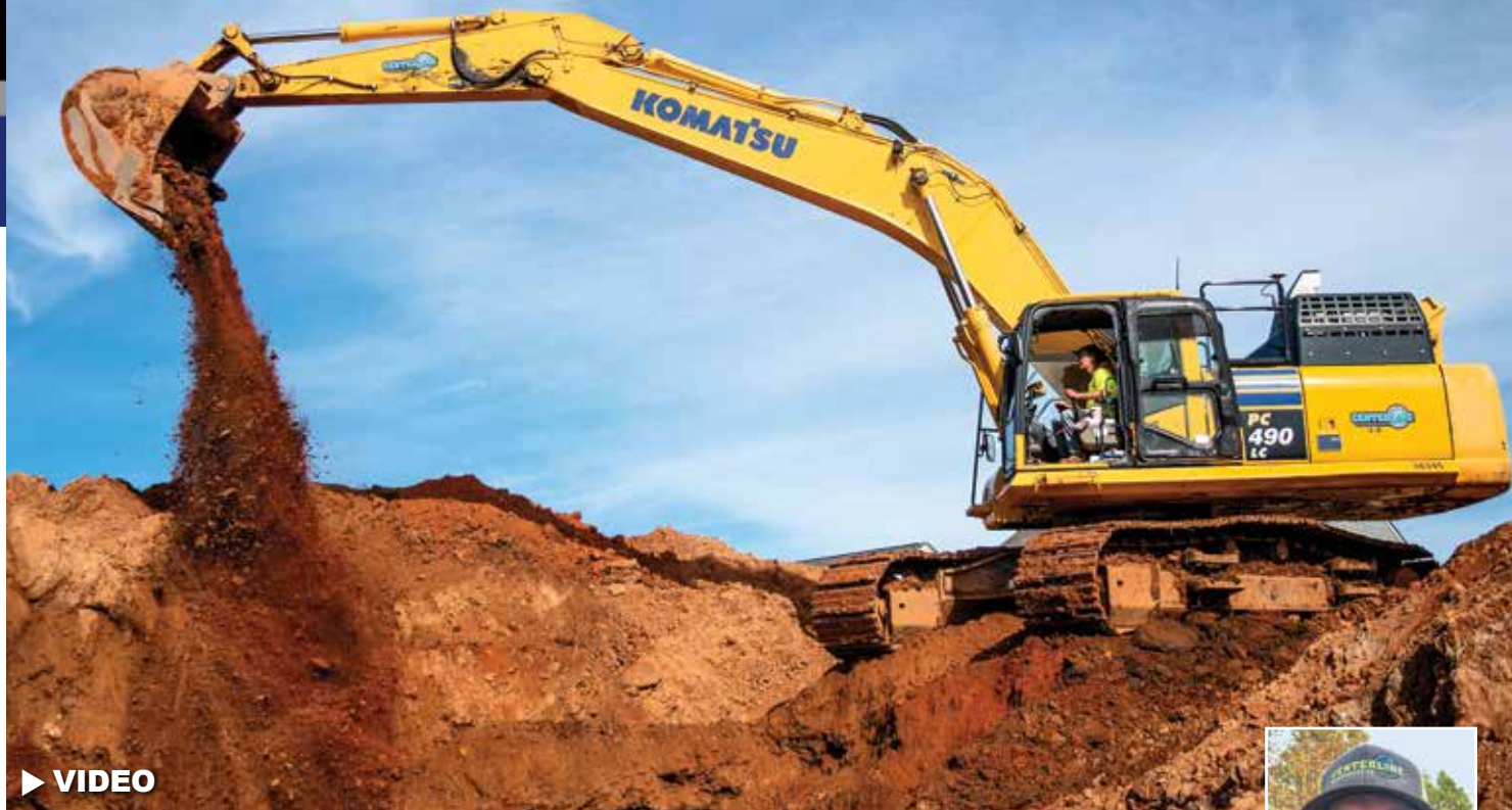
At a jobsite north of Charlotte, N.C., a Centerline Contractors operator moves dirt using a Komatsu PC490LC-11 excavator. "The machine has great swing time and lots of power, which allows us to move earth at a higher rate," noted Equipment Manager Mark Brantley. "It's excellent for mass excavating and larger jobsites like this."
