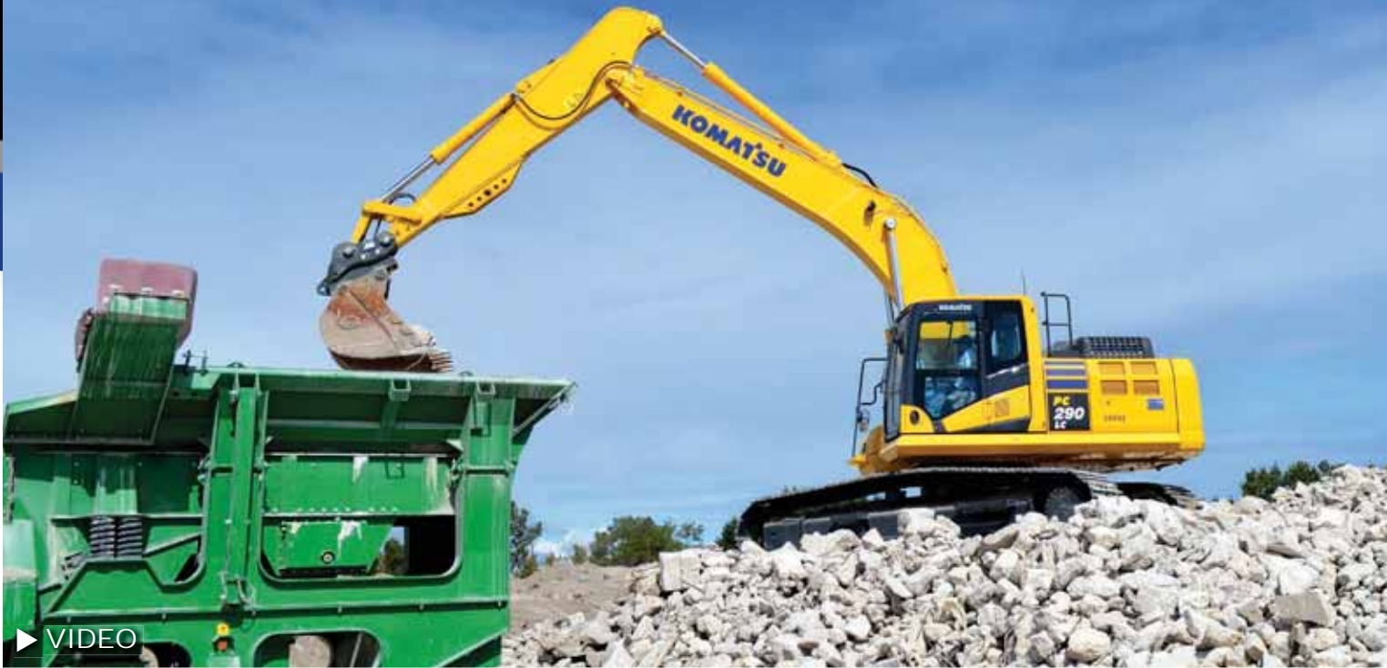
A Robcor operator uses a Komatsu PC290LC excavator to load a crusher at the former Splendid China theme park southwest of Orlando. The crushed rock will be recycled and left on-site for the park's new owners to use on infrastructure and road construction. Robcor will process nearly 200,000 tons of material during the six-month project.
