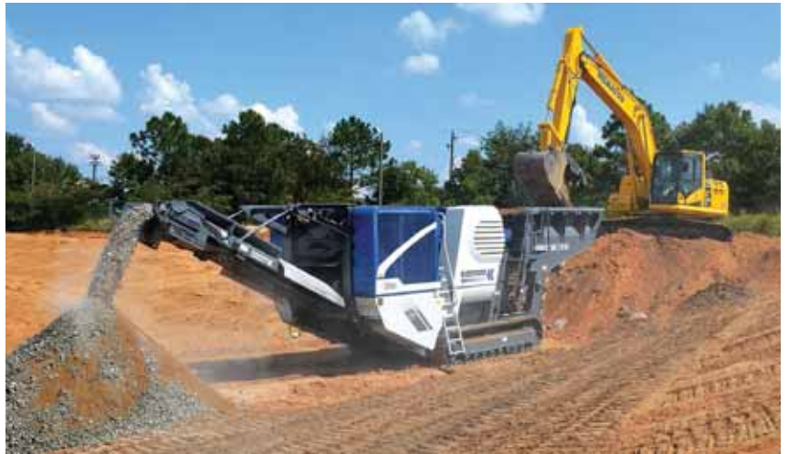
Attendees at the South Carolina Oktoberfest got to watch a demonstration of a Komatsu PC210LC-10 hydraulic excavator feeding the new Kleemann MC 110 Ri mobile impact crusher.
