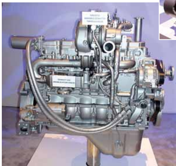
Komatsu displayed the technology behind its Tier 4 Final engines, including the selective catalytic reduction components (inset) that reduce emissions to near zero.
