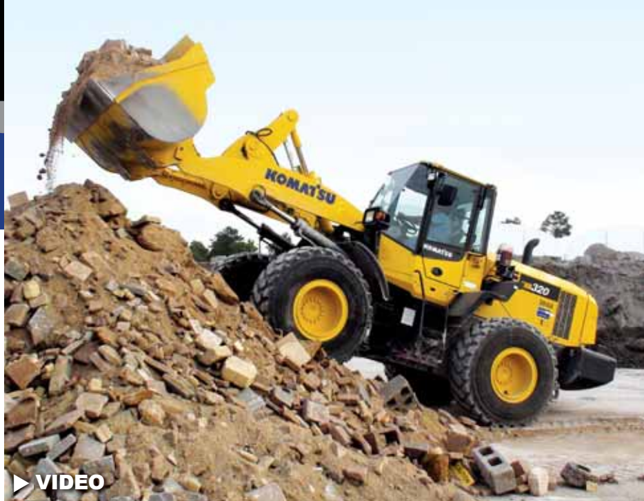
B.E.T.-ER Mix owns seven Komatsu WA320 wheel loaders including this new Dash-7 model. "We've always been pleased with the fuel efficiency of our WA320s, but the Dash-7 takes it to a new level, using 15 gallons per day less than the Dash-6," said owner Terry White.
