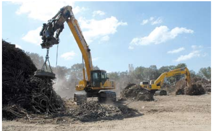
Four of Kuei Tyan's Komatsu PC400s are equipped with generators that power magnets to handle, move and load rebar and cable scrap.
