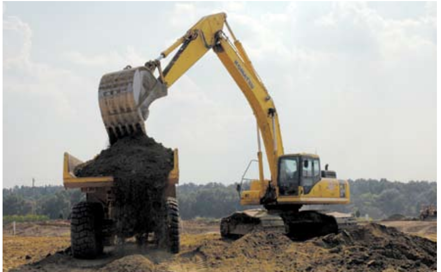
A Hoopaugh operator uses a PC300HD-7 excavator to load trucks at the Marvin Creek project in Marvin. "They are a good match for our 30-ton trucks," Larry Hoopaugh said of the 81,820-pound machines.
