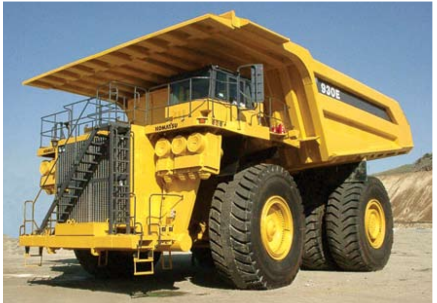
Komatsu's Peoria, Ill., plant heads up the manufacturer's worldwide R&D efforts for large mining trucks like the 330-ton 930E.
