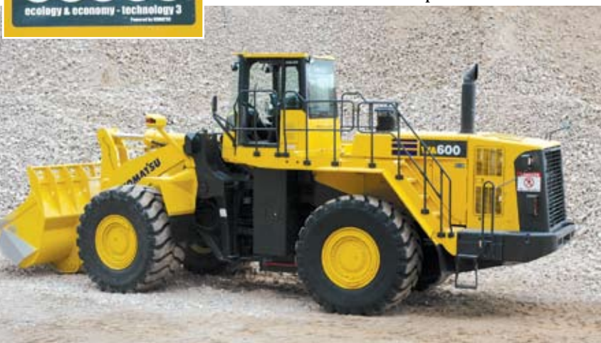
All new Dash-6 Komatsu wheel loaders, like the WA600-6 shown here, as well as all new Dash-8 excavators feature the new ecot3, Tier 3-compliant engine, which lowers both emissions and fuel consumption.
